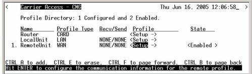
3. Select **Setup: <Static/VPN Networks>**, scroll with the **[SPACEBAR]** to through the options and select **[ENTER]**.
